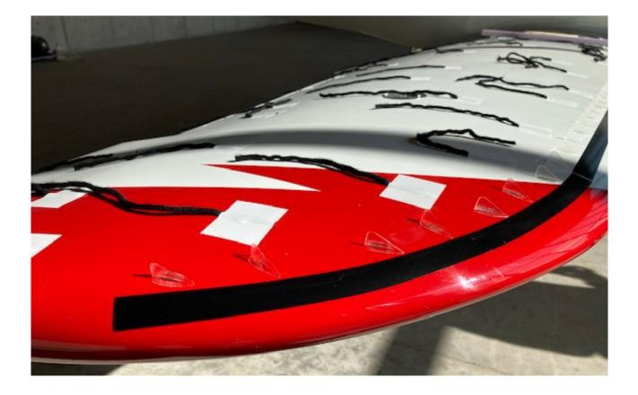
In addition we mounted a row of VGs underside the elevator with 30mm distancing and 100mm in front of the hinge. As with many airplanes the elevator is too small and has too little effect when landing at low speeds.
