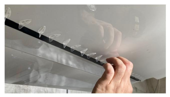
The second test flight with VGs only on the outer half of the wing, in front of the aileron, was a complete success. The plane remained fully controllable until full stall and the stall speeds were already much lower in all configurations.
