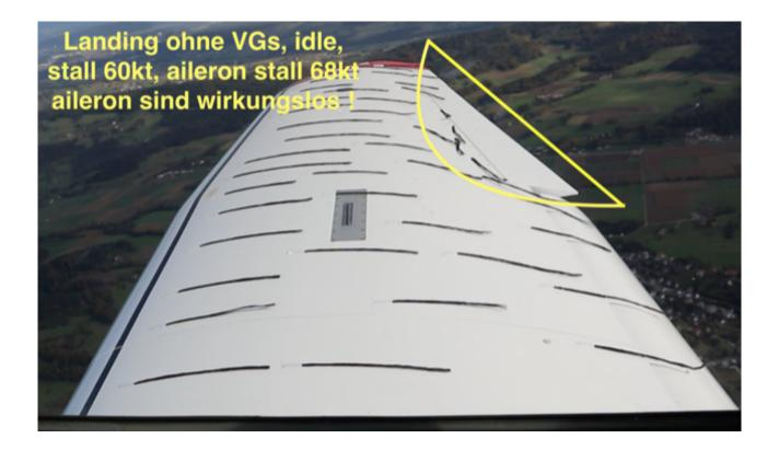
It became clear to me during the first stall attempt why Lancair pilots force their aircraft onto the runway for landing without flare to reduce the speed. **The aileron is wrongly constructed and stalls below 80kt.**
