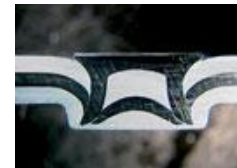
Aluminium 1,2 mm Stahl 1,0 mm Aluminium 1,2 mm
