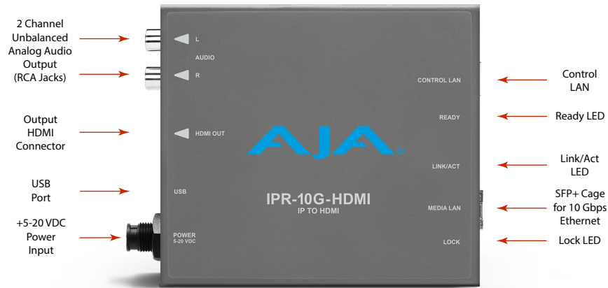
Figure 8. IPR-10G-HDMI Connections
