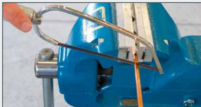
Determining the length of the pipe section. Here the additions for bends and flanges must be taken into account. Sawing off the pipe.
