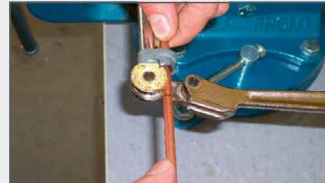
Inserting the pipe into the bending device
