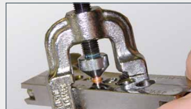
Flaring of the pipe with the flaring tool
