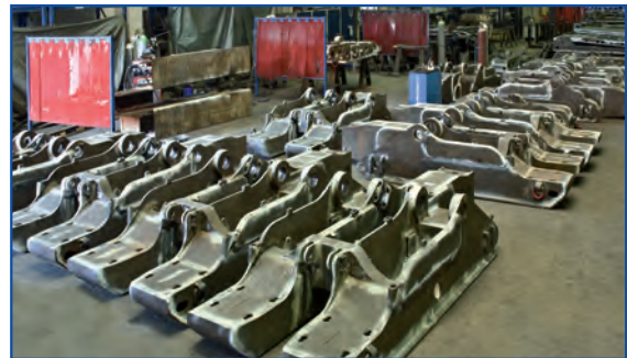
Refurbishing shield supports
