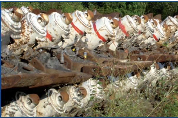
Used shield support units in outdoor storage
