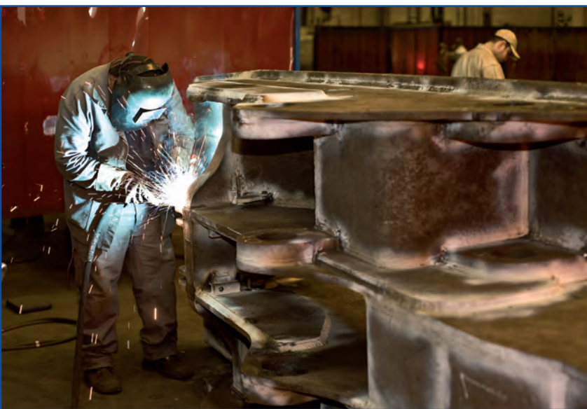
Refurbishing shield supports
