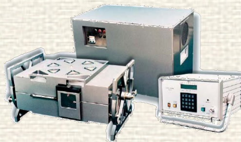
Portable 6 MeV betatron for radiography
