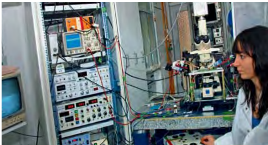
A student, Rebecca Böhme, performing patch clamp recordings of cerebellar nuclei neurons in live brain slices.
