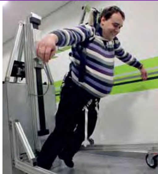
The displayed system allows the application of external mechanical perturbations to the body in order to study the motor control during complex walking
