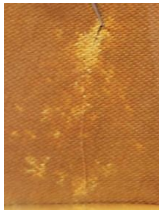
Figure 2: White Mark on Pressboard Surface
