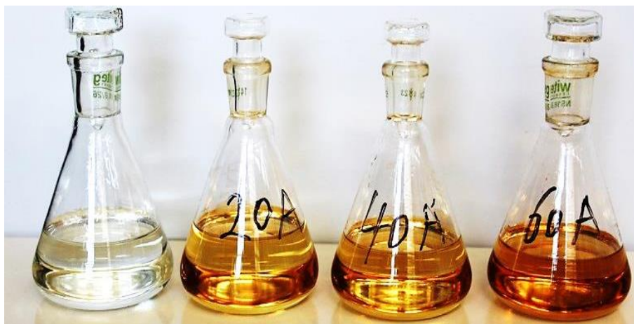
Figure 3: The oil/pressboard samples of different ageing degrees (from left to right: new, 20 days, 40 days, and 60 days)
