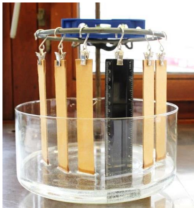
Figure 1: Capillary Water Rise Test of pressboard
