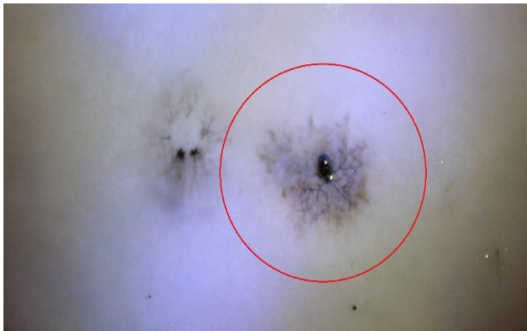
Figure 2: The effect of very high electrical stress on the surface of the aramid pressboard (surface discharge) at 1.5 nC average apparent charge
