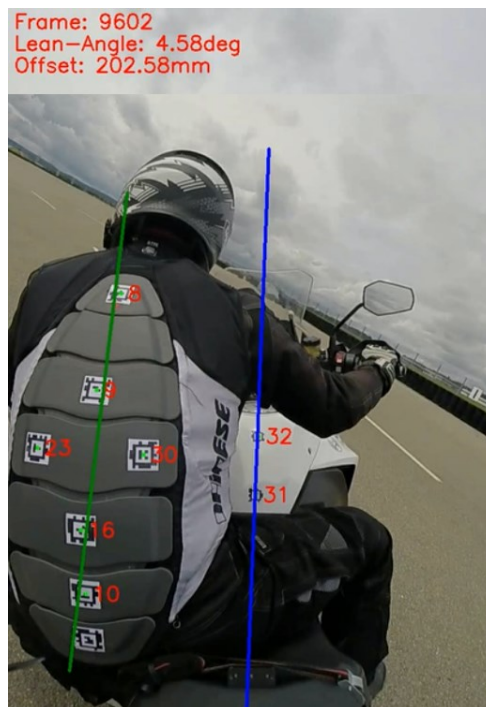
Fig. 1. Marker based optical measurement system for rider upper body position using AprilTags. Rider upper body lean angle and lateral offset are calculated relative to the motorcycle centreline (blue). The rider centreline (green) is calculated with linear interpolation using all AprilTags that are detected along the rider's spine in a single frame. The individual numbers of the markers that are successfully detected are depicted in red beside them.
