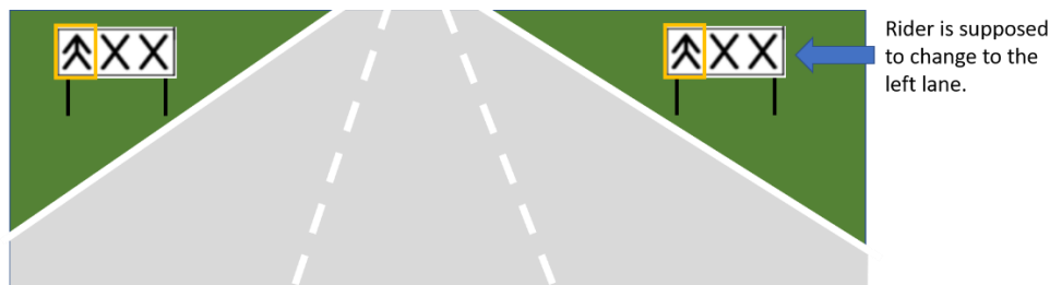
Figure 4: Schematic representation of the LCT and the signs indicating the next lane change (in this case to the left lane).
