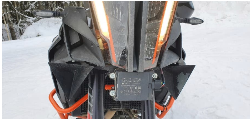
Figure - The radar (in centre) and radar reflectors on Connected Motorcycle JARNO ©VTT.
