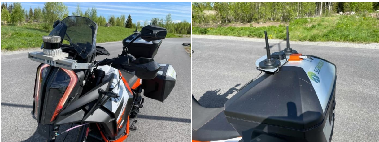
Figure – JARNO - The Connected Motorcycle Platform of VTT. Front: LiDAR and radar (left); Rear LTE-4G/G5 comms antennas, IMU, GNSS (right) ©VTT
