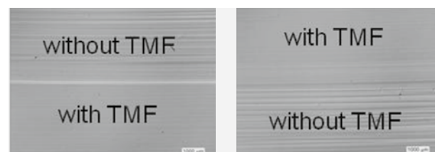
Fig. 1 Detail of DSL-etched longitudinal cuts of Si-doped GaAs VGF crystals grown with and without TMF influence.
