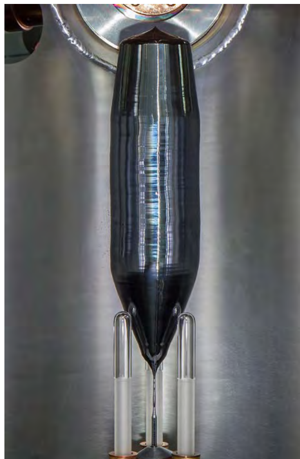
Fig. 1 ^{28}\text{Si} dislocation free single crystal grown by FZ technique
