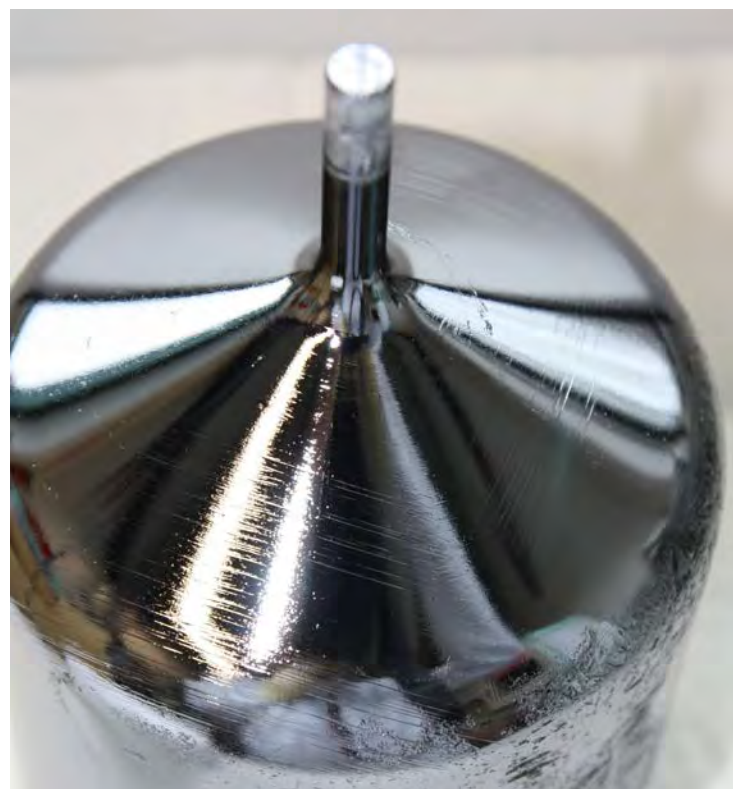
Fig. 2 Image of 4 inch GaAs VGF single crystal with strong facets.
