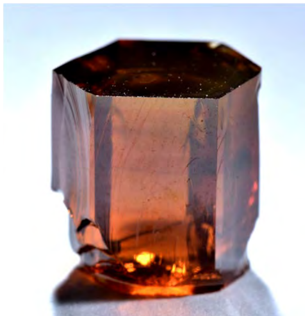
Fig. 6 AlN single crystal grown by sublimation/recondensation, maximum 10 mm \emptyset , diameter enlargement from 8 mm to 10 mm.
