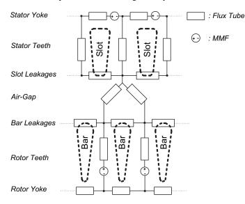
Fig. 1. Permeance network model for a portion of a SCIM
