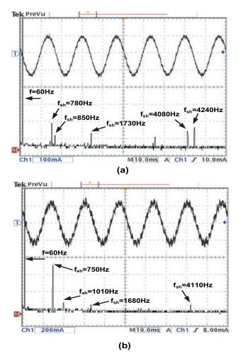
Fig. 4. FFT of the stator current  $(\frac{A}{100})$  during (a) no-load and (b) loaded steady-state operations obtained from the linear PNM model
