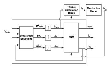
Fig. 2. Schematic diagram of a SCIM model
