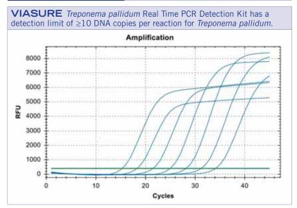
Dilution series of Treponema pallidum (10<sup>7</sup>-10<sup>1</sup> copies/rxn) template run on the Bio-Rad CFX96™ Real-Time PCR Detection System (channel FAM)
