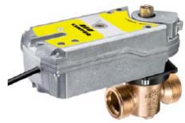
KHS-VAV maximum flow isolating ball valve with servo drive and spring reset Figure 686 05 230 V AC Figure 696 05 230 V AC (Discharge water limited max. 2 l/min)
