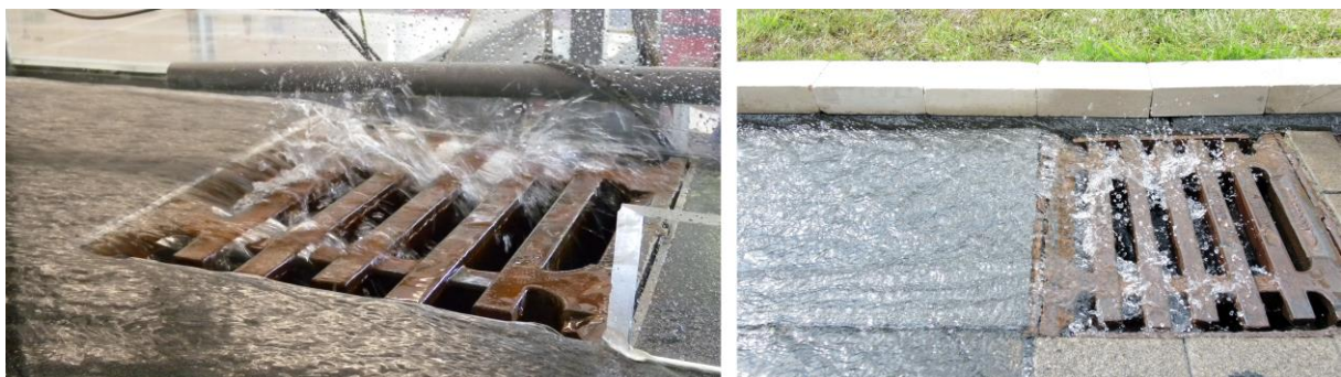
Abbildung 55: DIN 19583, Q = 9 l/s (links: Labor ( S_L = 5\% ), rechts: Feld ( S_L = 6\% ))
