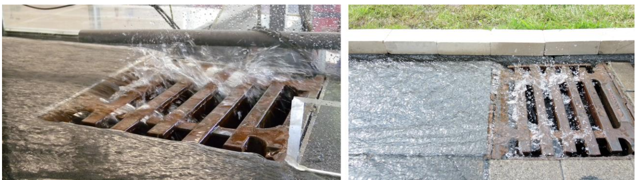
Abbildung 9: DIN 19583, Q = 9 \text{ l/s} (links: Labor ( S_L = 5 \% ), rechts: Feld ( S_L = 6 \% ))
