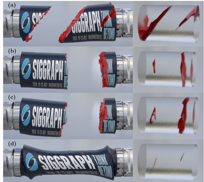
Fig. 2. Tube Pull. We stretch a 45 degree fibered tube and show its material space for (a) anisotropic damage and anisotropic elasticity, (b) isotropic damage and isotropic elasticity, (c) anisotropic damage and isotropic elasticity, and (d) no damage and anisotropic elasticity. This illustrates the strength of coupling anisotropic damage with anisotropic elasticity, as only one or the other method leads to weakly guided fracture (c) or numerical fracture (d). Note that (d) does eventually fracture, but it is uncontrollable and numerical.
