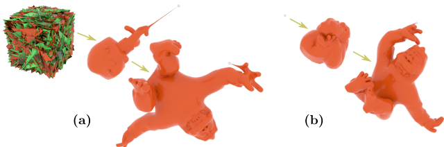
Fig. 19. Inversions and Extreme Deformations. We use mesh-based linear FEM to show that our QR-elasticity is robust under extreme circumstances. We show that both (a) a randomly initialized configuration and (b) a one-point initialized configuration can recover the rest shape of the gorilla and model accurate dynamics (assuming the absence of plasticity).
