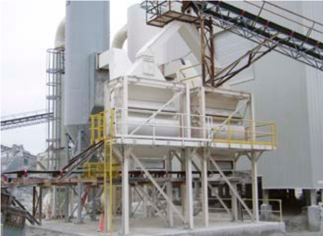
Two AC 27 working in parallel with a joint capacity of 150 tph.
