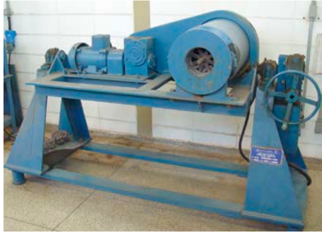
12"x24" Rod mill (Bond rod mill) Twin pendulum breakage device.
