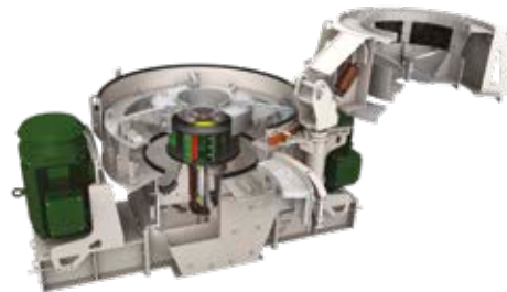
Impactor (VSI) rock-on-rock action
