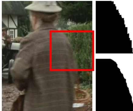
Figure 11.5: Difference between a discrete (top) and a continuous model (bottom). The discrete model shows block artifacts since its discretization error does not converge to 0 for finer grids sizes.
