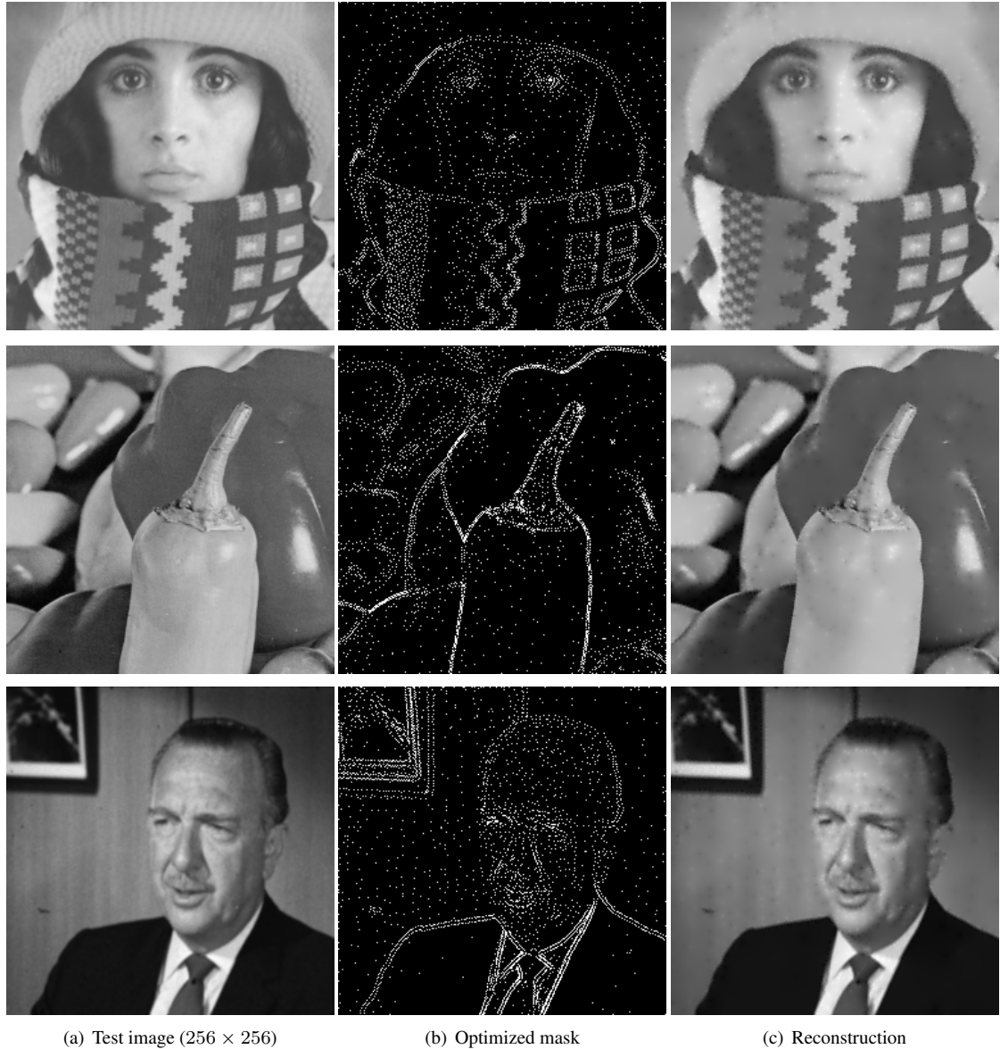
Figure 6.7: Examples of finding optimal inpainting mask for Laplace interpolation based image compression by using iPiano. FIRST ROW: Test image trui of size 256 \times 256 . Parameter \lambda = 0.0036 , the optimized mask has a density of 4.98% and the MSE of the reconstructed image is 16.89. SECOND ROW: Test image peppers of size 256 \times 256 . Parameter \lambda = 0.0034 , the optimized mask has a density of 4.84% and the MSE of the reconstructed image is 18.99. THIRD ROW: Test image walter of size 256 \times 256 . Parameter \lambda = 0.0018 , the optimized mask has a density of 4.82% and the MSE of the reconstructed image is 8.03.
