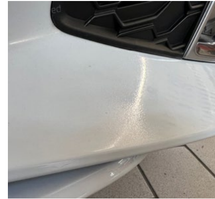
Mangelhafte Lackreparatur (Spotrepair)
