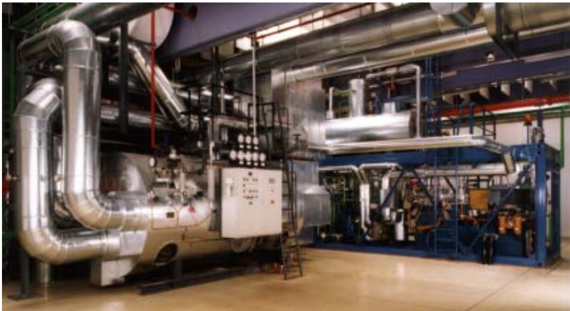
Figure 41: Prototype plant for a steam screw-type engine at the University of Dortmund
