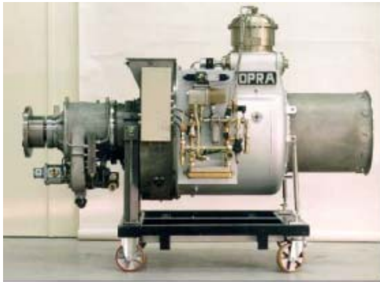
Figure 13: Gas turbine FP-16-G
