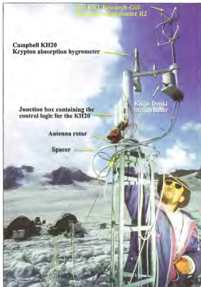
Figure 2: System for eddy correlation measurements, which is mounted on a 2 m tower and run continuously during 5 day periods in August 1998 and 2000, respectively, at Vernagtferner (Oetztal Alps, Austria) at an elevation of 3000 m a.s.l. The glaciologist is Markus Weber, the author. (Picture by Jan Greune)
