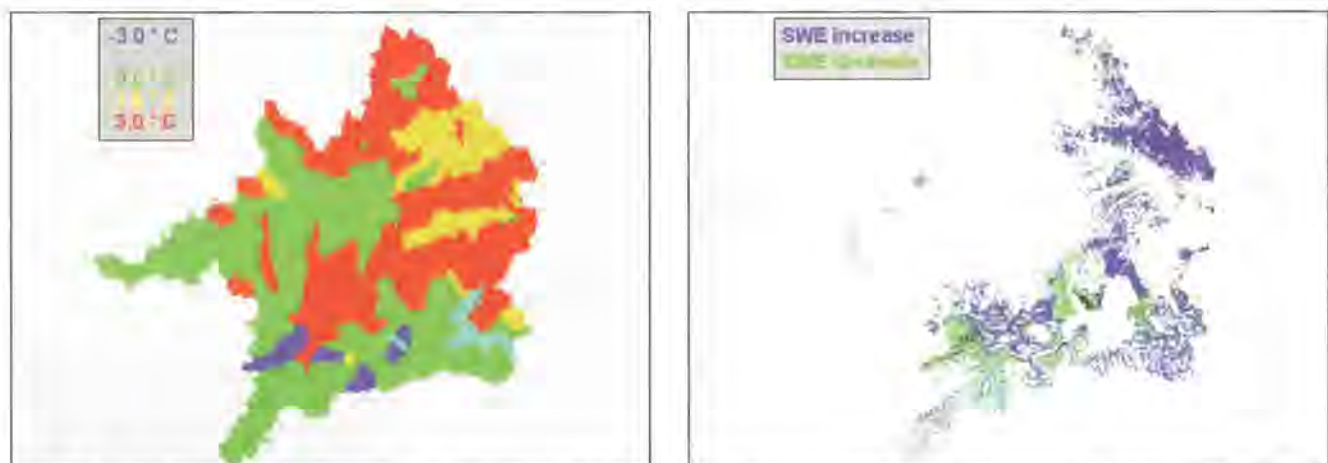
Figure 6: Distribution of estimated critical temperatures in the catchment for a snowfall period (12.2.-18.2.2006) derived from comparison with snow maps observed with satellites (left) and resulting increase or decrease of simulated snow water equivalent (right).
