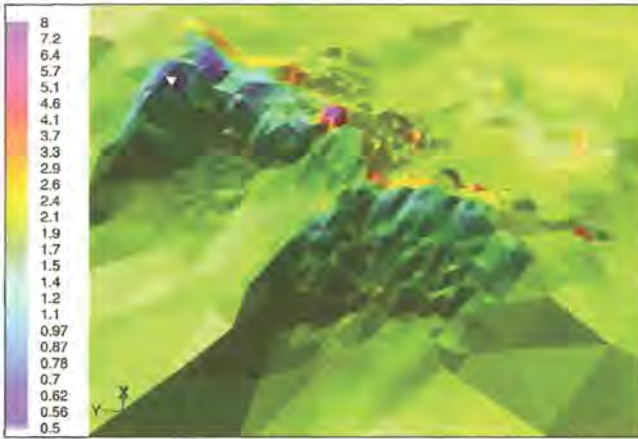
Figure 9: Snow drift pattern at the upwind side of the mountain ridge. The color bar corresponds to the snow depth in m
