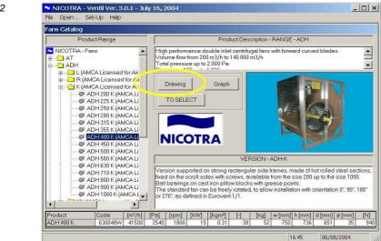
The **Drawing** button opens a new window showing the fan dimensional drawing, with the principal dimensions, like the following example:
