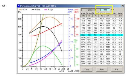
On the right side of this new window there is a table listing the fan performance curves at the specified speed (shown inside the text box on top of the window). You can see values for Flow Rate, Static Pressure, Dynamic (Velocity) Pressure, Total Pressure, Mechanical Power, Total (Mechnical) Efficiency and Sound Power Level. The line with the original duty point is highlighted with a light blue backgroud.
