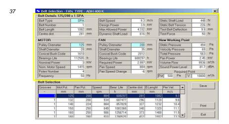
The numerical data in the top highlighted region refers to the belt drive selected in the lower grid. If you select a new line, all the numerical data will change, according with the new selected drive. Again, pressing the key combination Ctrl-C copies the belt selection data into the clipboard, so you can paste them into a document or a spreadsheet.
