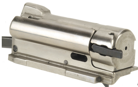
The bolt is unchanged from previous Golds. The locking lug at the bolt's rear engages a recess in the barrel extension. A hook extractor is on the bolt's right.
