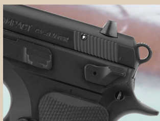
The new double-action P-01 has a decocking lever on the frame's left rear. The frame is of aluminum alloy, and the lanyard ring on its bottom reflects its origin as a Czech National Police arm.
