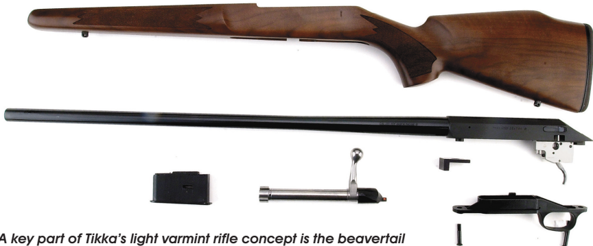
A key part of Tikka's light varmint rifle concept is the beavertail fore-end with a flat bottom for shooting from a rest. However, the fore-end remains narrow enough for comfortable position shooting in the field. The result is a fully capable, portable rifle.
