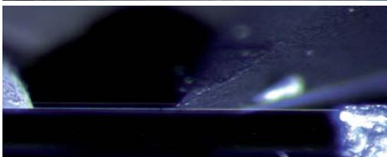
Diamond knife approach as seen through the Leica M80 stereo-microscope with backlight illumination.
