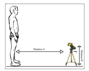
**Figure: 7.** Distance A between tibia and IR Camera: 240 centimeters. Distance B between ground and midpoint of camera lens: 51 centimeters.
