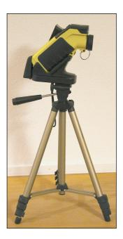
Figure: 5. Infrared camera and its tripod
