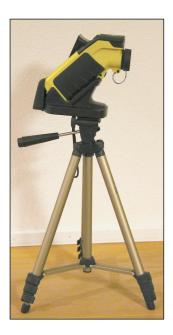
Figure: 8. Infrared camera and its tripod
