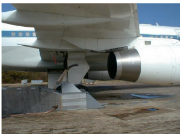
Figure 1. Langley B-757 with test stand and probes positioned 1 meter behind engine exhaust plane.
