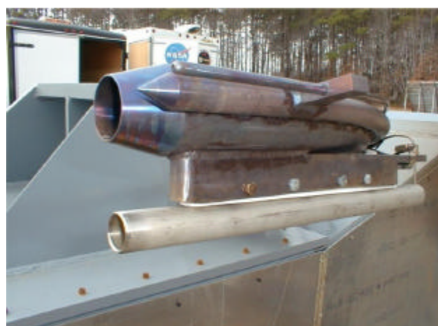
Figure 2. Gas and aerosol inlet probes along with pitot tube and Gerdien Condenser used in 1 and 10 meter sampling behind the B-757.
