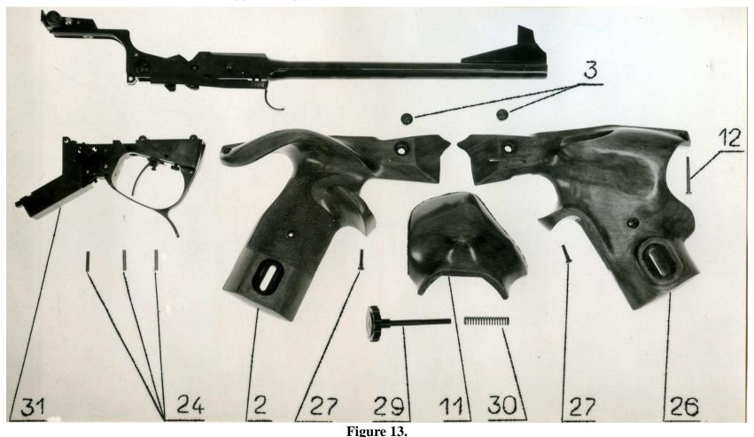
2 – right cheek; 3 – nut; 11 – palm rest; 12 – grip screw; 24 – connecting pin; 27 – grip screw; 29 – palm rest screw; 30 – sprint of palm rest screw; 31 – striking & trigger mechanism;
