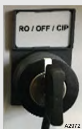
Schlüsselschalter RO/ OFF / CIP
