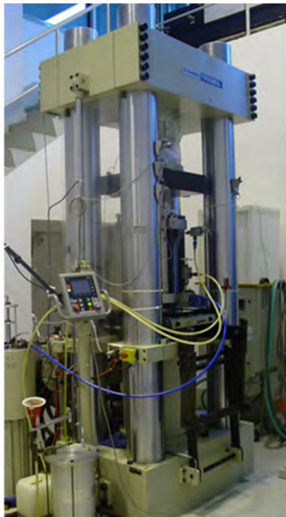
Figure 1: Servohydraulic testing machine and experimental setup for permeability measurements. Flow rates are measured at the top (labelled by q_0 ).
