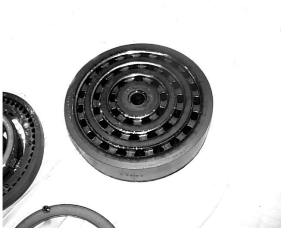
Picture 5: Ring type valve showing signs of liquid in gas stream. This was identified by condition
