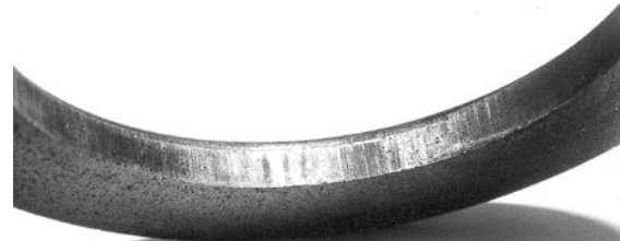
Figure 7. Radial wear opposite the gap of throttle ring
