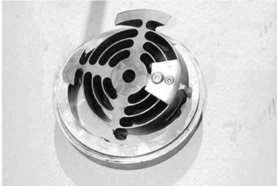
Picture 2: Damaged suction valve following liquid carry-over.
