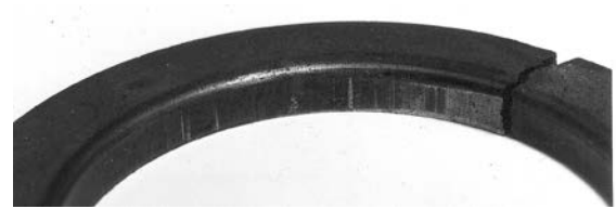
Figure 6. Radial wear beside the gap of throttle ring
