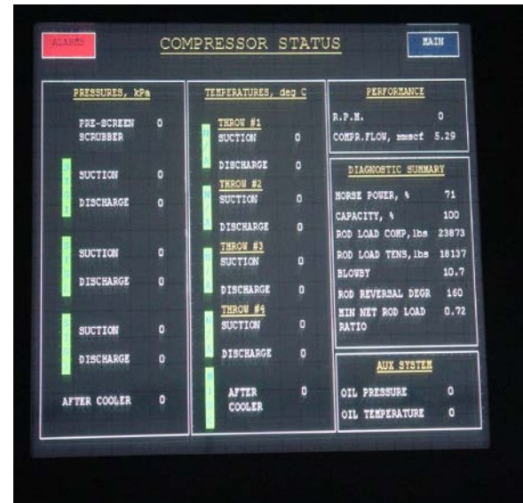
Picture 2.1: PLC panel Sentry Pro* by Prologix Controls of Calgary, Alberta, Canada, using the ENALYSIS Diagnostic Software.
