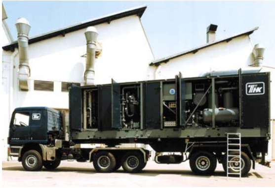
Picture 2: Containerised Nitrogen Generation System (Truck Mounted)
