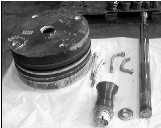
Figure 1: Damaged piston parts
