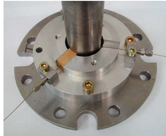
Fig. 3: Measurement of rod temperature by sliding contact of three insulated thermocouples.
