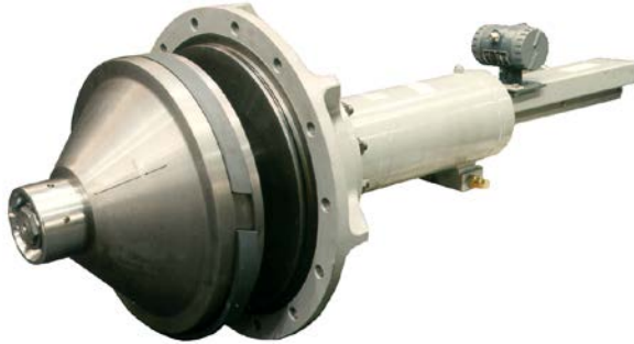
Figure 3: Conical piston and hydraulic cylinder
