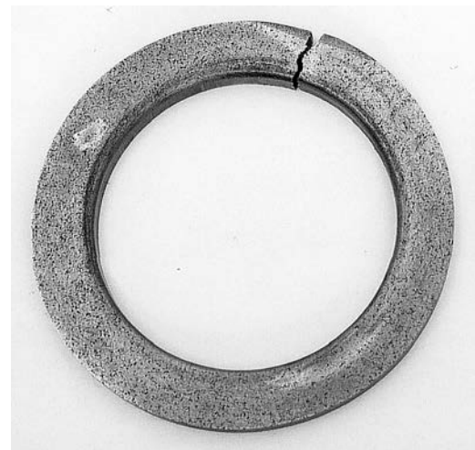
Figure 8. Axial wear of seal ring
