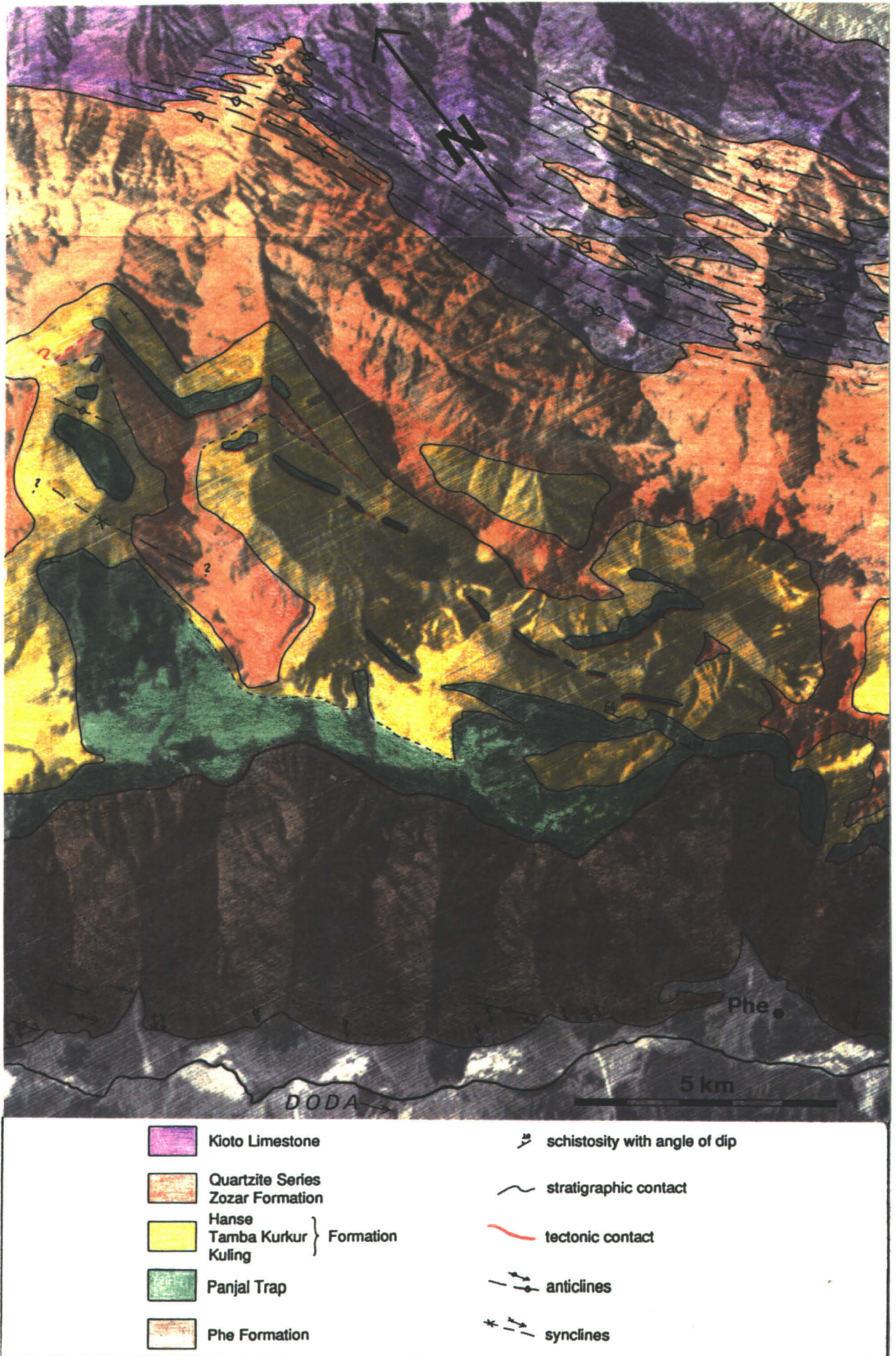
Figure 3.21: Detailed geological scetch map of the Ralakung region showing the individual Panjal Trap thrust sheets.
