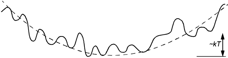
Figure 4.54: Model of a two-dimensional cut through the energy hypersurface of an amorphous material
