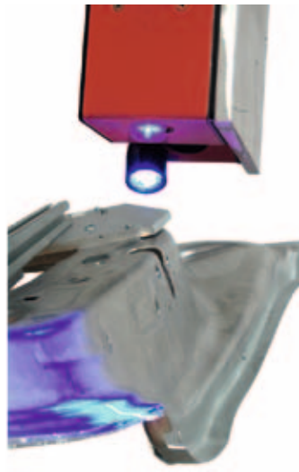
Middle and right: Weld Seam Inspection with one sensor.
