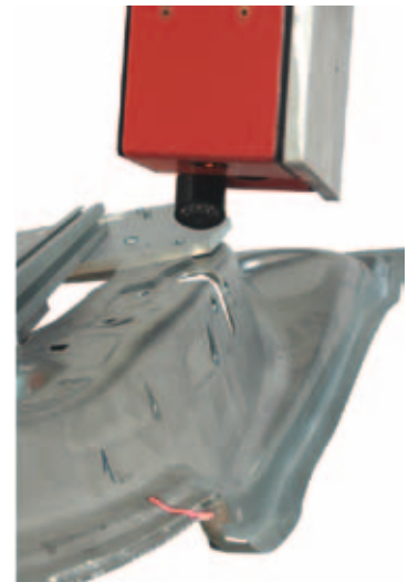
Middle and right: Weld Seam Inspection with one sensor.
