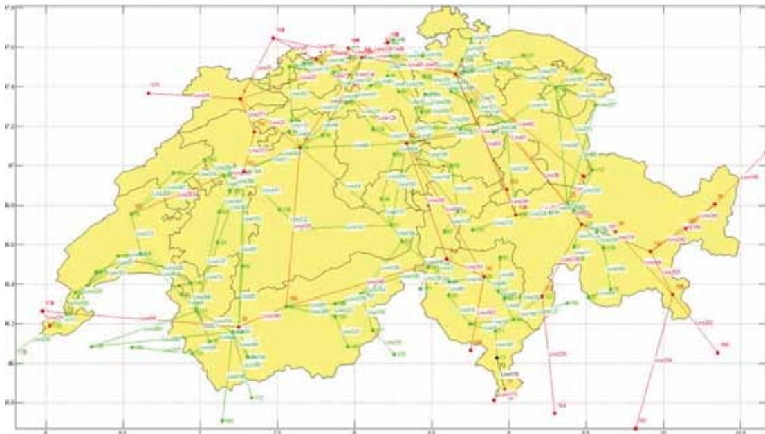
Figure 3 – Transmission Grid of Switzerland (Plan for year 2020) – green: 220 kV, red: 380kV (Reproduction from Swissgrid grid model data).
