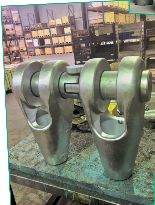
George Washington Bridge Socket (GWBS)
