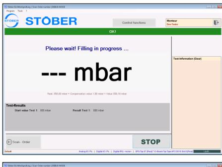
In the second step, the software automatically performs the leak test with the help of the PLC.
