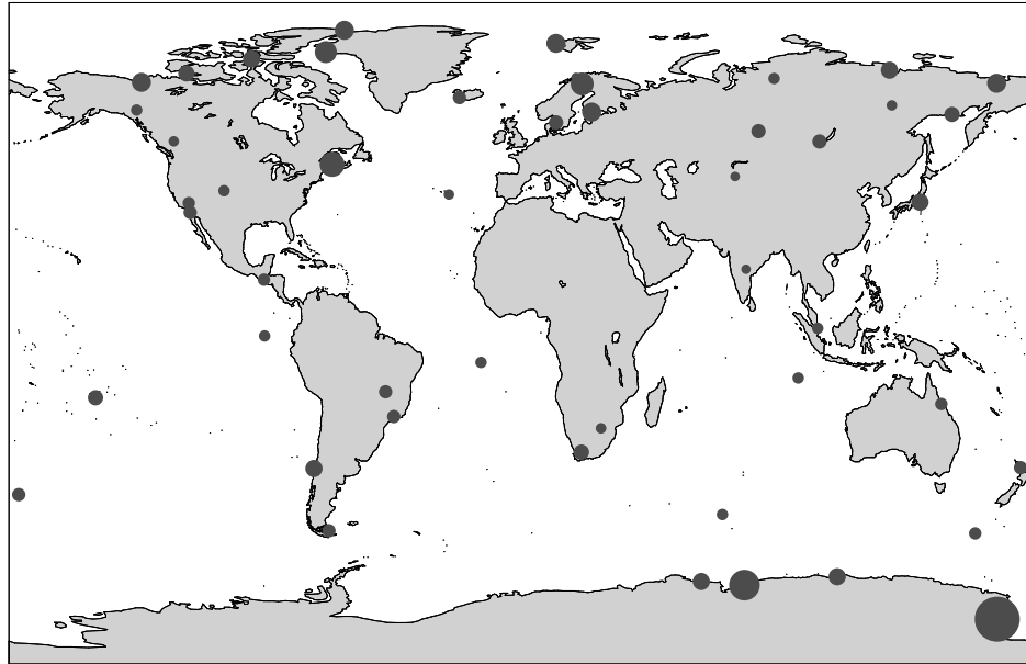
Figure 8.2: Globally distributed IGS stations used for GRACE orbit determination on DOY 250, 2003. The diameter of the circles is proportional to the incidence of a maximum number of simultaneously observed GPS satellites with the GRACE A BlackJack receiver.
