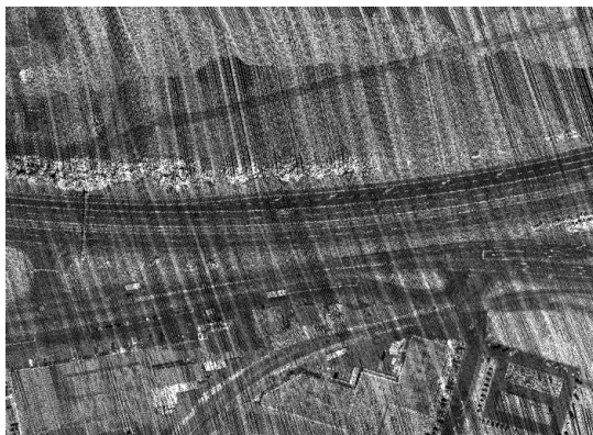
FIG. 2.6: Point-cloud colored by non-normalized intensity values.
