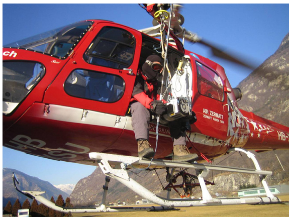
FIG. 6.1: Scan2map-system suspended on the winch of a helicopter.
