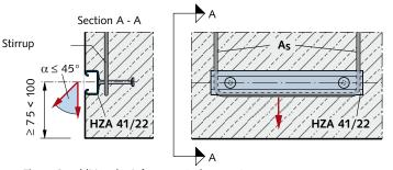
Figure 2: additional reinforcement placement
