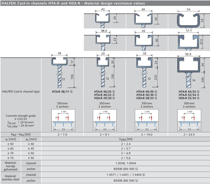
② Material 1.0038, ③ Material 1.0044, ④ Not available for HALFEN Cast-in channels HZA-R 29/20 **Notes:** HALFEN Cast-in channels HTA-R / HZA-R are not included in the HTA-CE / HZA-Approval
