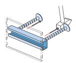
Where possible, use stainless steel nails to avoid corrosion.
