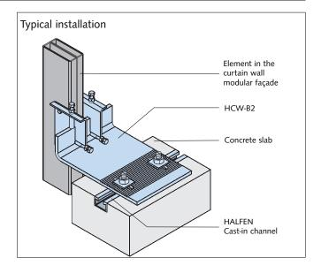
The façade planner is responsible for providing the static verification for the support posts. Use HALFEN Bolts M16 Grade 8.8 (order separately), to connect the base bracket to the HALFEN Cast-in channel. Depending on the façade type, the connection between the connecting plate and the base bracket can be designed either laterally adjustable or as a fixed point.
