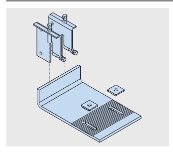
HALFEN Brackets HCW-B2 are made in grade S355 quality galvanized steel. The vertical adjustability is  $\pm$  24 mm. Three dimensional adjustability is ensured when used in combination with HALFEN Cast-in channels HTA-CE.
