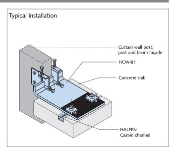
The lateral connecting plates are connected to the façade posts using M8 screws (not included). The façade planner is responsible for providing the static verification for the support posts. Use HALFEN Bolts M16 Grade 8.8 (order separately), to connect the base bracket to the HALFEN Castin channel. Depending on the façade type, the connection between the connecting plate and the base bracket can be designed either laterally adjustable or as a fixed point.
