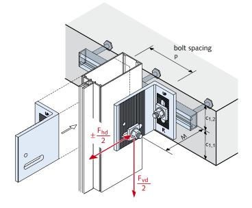
To guarantee correct installation, the HCW-ED brackets are marked 'R' for right, 'L' for left and 'UP' for top.
