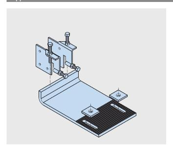
HALFEN Brackets HCW-B1; for installing to the top of concrete slabs, are available in two load ranges and three cantilever sizes. The brackets are made in grade S355 quality galvanized steel. Vertical adjustability is  $\pm\,10\,\text{mm}$ . Three dimensional adjustability is ensured when used in combination with HALFEN HTA-CE Cast-in channels.
