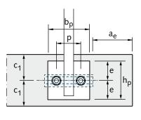
$<sup>\</sup>textcircled{1}$  e = distance between anchor channel axis and outer edges of the anchor plate. For asymmetrical anchor plates the smallest distance to the outer edge of the anchor plate is used for calculation.
