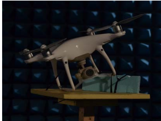
Fig. 6. Measurement setup for tilted (roll 28 degrees) Phantom 4.
