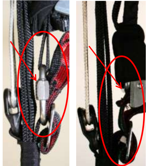
locked trimmer free trimmer
