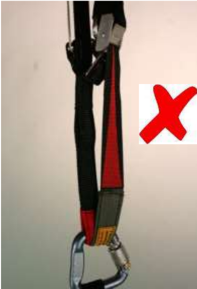
Fig. 11: Trimmer loop in the main carabiner
