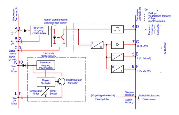
Attention: When several analog outputs are used simultaneously, each output requires a separate ground wire to be installed directly close to the sensor.
