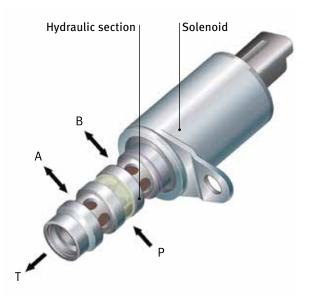
The control valve is a proportional valve with four connections, with one connection each to the:
