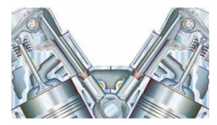
The lower camshaft is mounted below the separation line of cylinder head and engine block. This design is called overhead valve (OHV).
