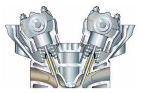
If two camshafts are mounted, the arrangement is called double overhead camshaft (DOHC).
