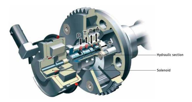
The central valve is a proportional valve with five connections, with one connection each to the:
