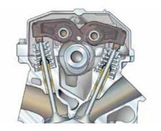
The upper camshaft is mounted above the separating line of cylinder head and engine block. With only one camshaft, this set-up is called overhead camshaft (OHC).
