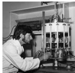
Measuring O 2 uptake using a Warburg apparatus – 10 ml incubations
