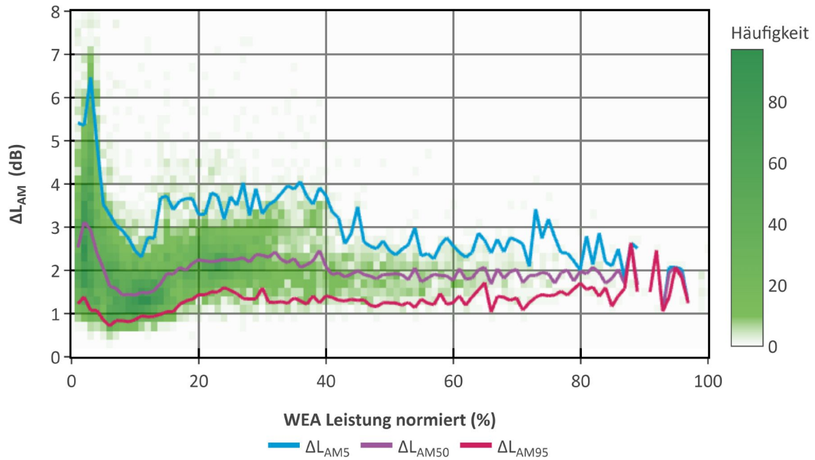
Figure 122: SA 1, emission, modulation depth of amplitude modulation (5, 50 and 95 percentile) and wind turbine output (standardised)
