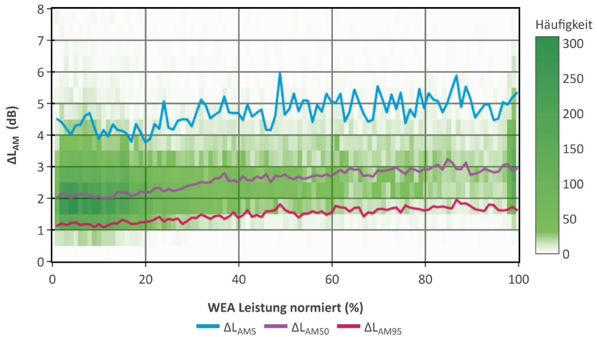
Figure 124: SA 2, immission, modulation depth of amplitude modulation (5, 50 and 95 percentile) and wind turbine output (standardised)
