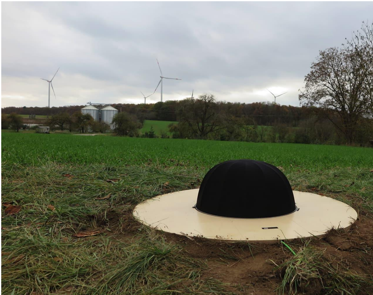
Figure 38: Infrasound microphone on ground plate
