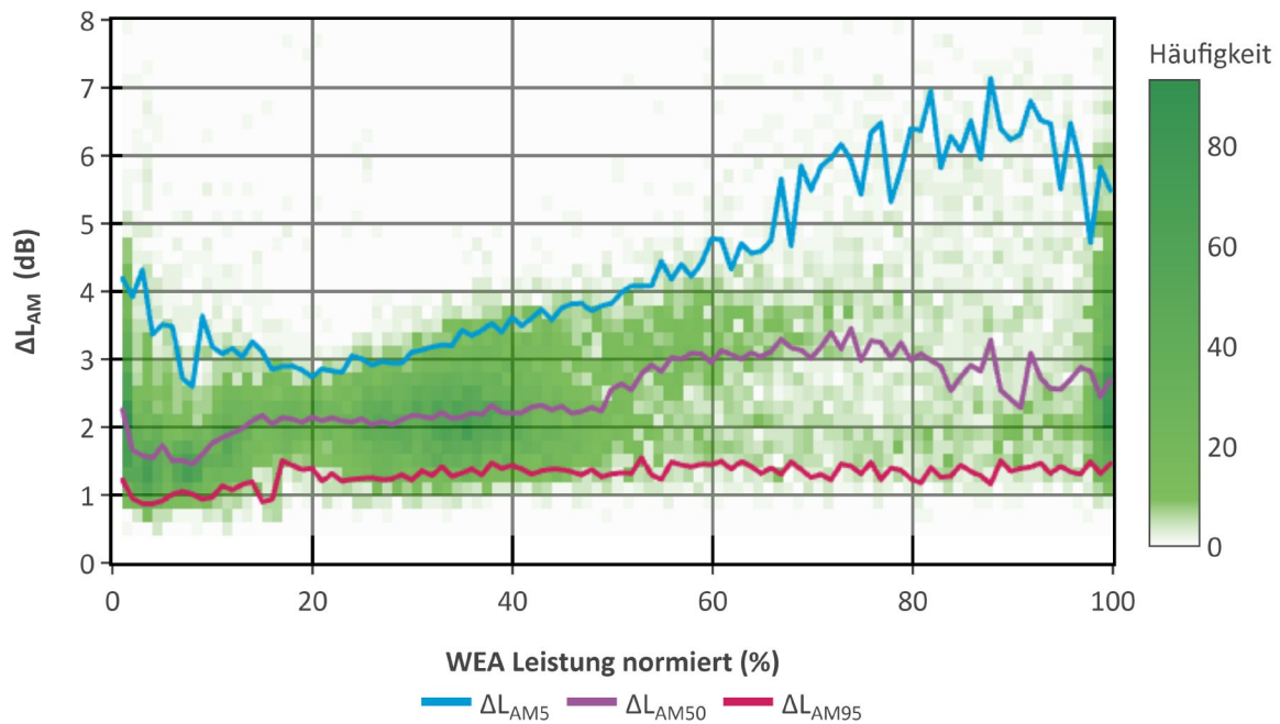
Figure 125: SA 3, emission, modulation depth of amplitude modulation (5, 50 and 95 percentile) and wind turbine output (standardised)
