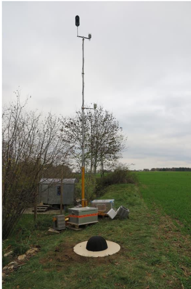
Figure 51: Measurement on the ground plate alongside measurement on a tripod
