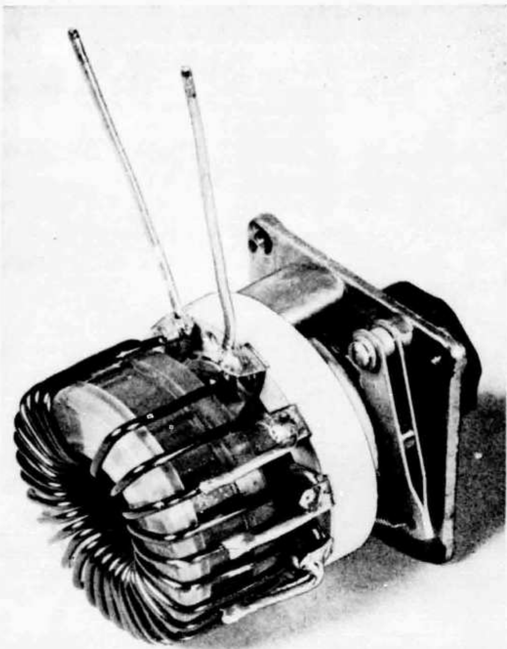
Fig. 7. Medium power (500 watt) toroidal tank coil employs one powdered iron core. The polystyrene end-spacers prevent flashover from the winding to the core. Coil taps for the various amateur bands are made to the outside of the windings that bridge across the two end spacers.
