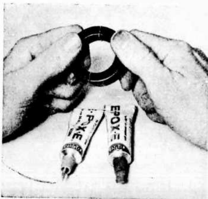
Broken powdered iron cores may be repaired with epoxy or household cement. Core material is a quasi-insulator and electrical contact between the broken pieces is neither required nor desired.
