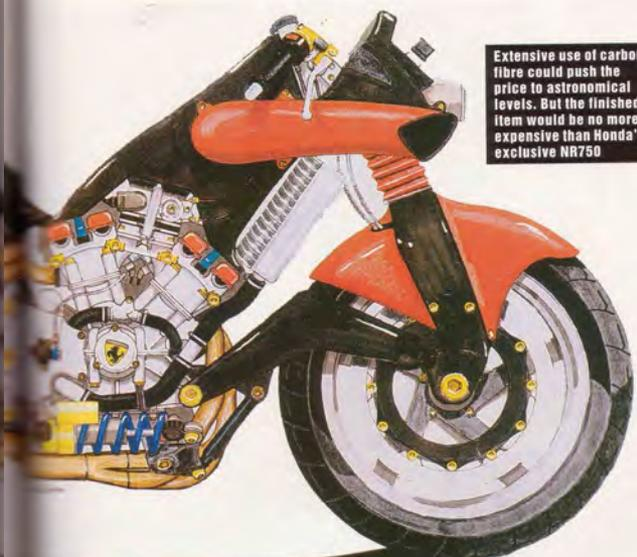
frame contains the silencers and inevitable catalyser. An air inlet leads cooling air through the rear sub-frame, and this has the additional effect of reducing noise too, although not too much of the beautiful eight cylindered melody is lost. Four chromed exhausts exit from the side of the seat hump.
