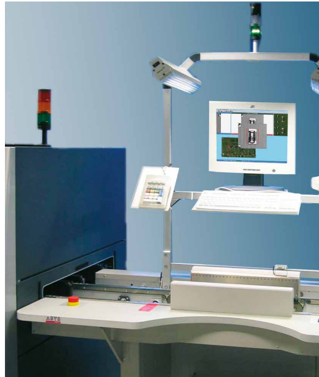
Verification station with separate handling module
