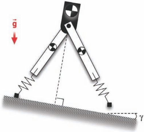
Fig. 1: A general passive dynamic walker model of locomotion.
