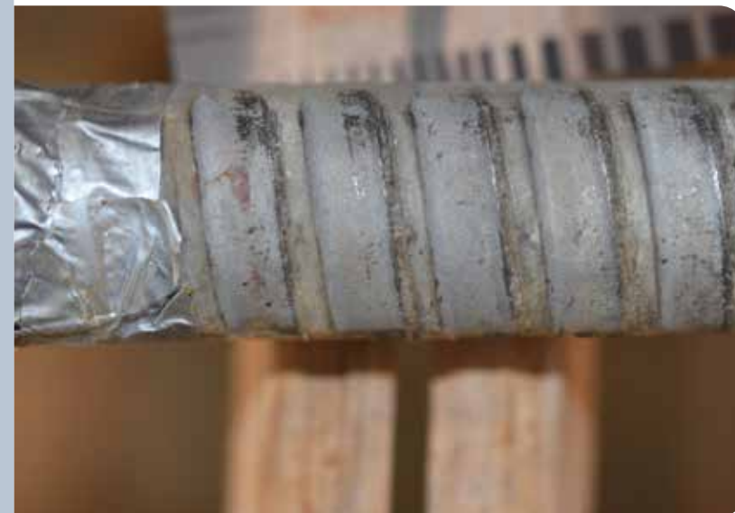
Figure 6: Other pictures of damages to micropiles; spacer (above); top of galvanized rods after unscrewing a sleeve (below)
