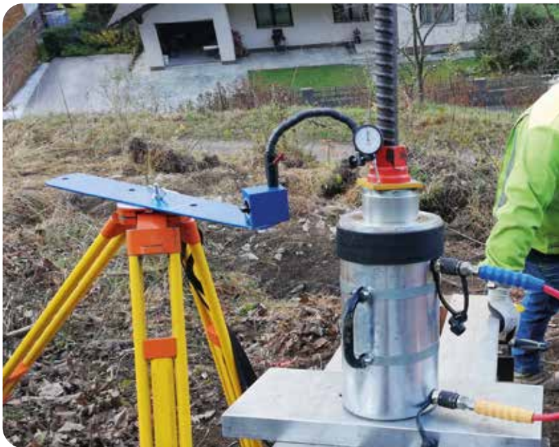
Figure 2: The two most frequently used methods of movement measuring: measuring cord orthogonal to the pulling device (picture above), tripod with dial gauge (picture below).
