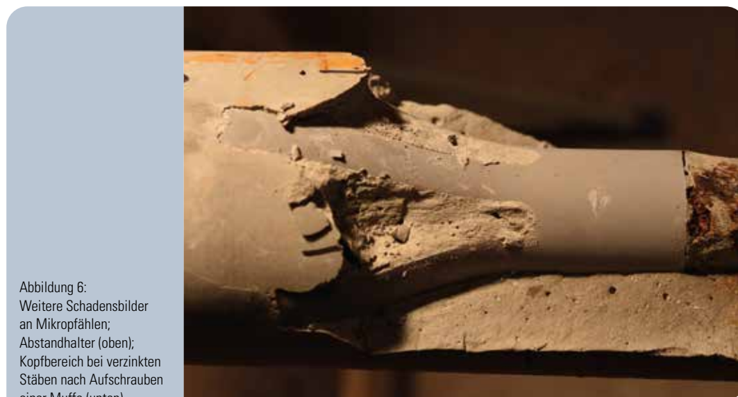
Figure 6: Other pictures of damages to micropiles; spacer (above); top of galvanized rods after unscrewing a sleeve (below)
